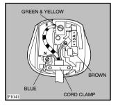
The wire coloured green and yellow must be connected to the terminal marked with the letter «E» or by the earth symbol  $\stackrel{\bot}{=}$  or coloured green and vellow.
